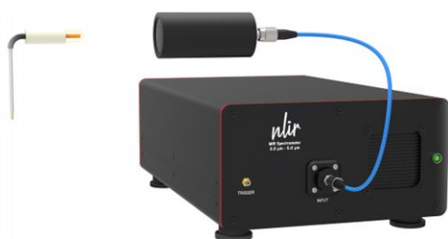
Schematic of an infrared light source and a fiber-coupled NLIR infrared spectrometer. A collimation tube is used to focus light from the light source into the fiber. The light source here is a hot blackbody-like filament, but it could be any infrared light source or hot object.
