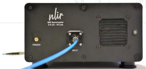
The NLIR S2050 MIR Spectrometer is based on a novel measurement scheme that upconverts the MIR light to near-visible light. Silicon-based near-visible light detectors are far superior to MIR light detectors in terms of detectivity, speed and noise. The NLIR upconversion technology therefore brings these attractive features, and the advantages that follow, to the MIR regime.
