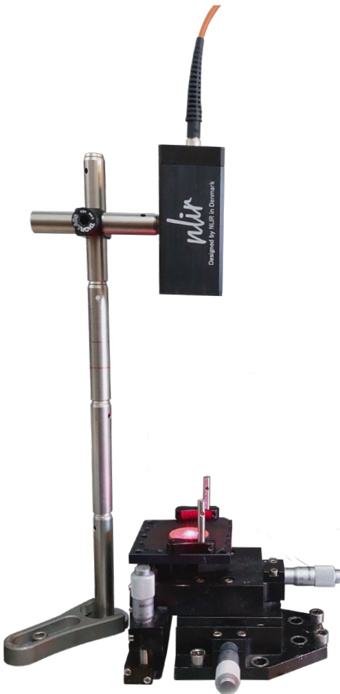
The SAMPLER Accessory collects light from the red spot on the translation stage.
